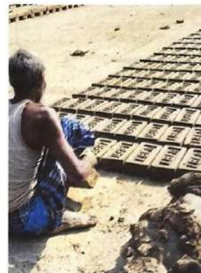
Brick making by clay at LBFA Brickfield
